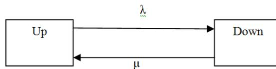
Figure 2: Two state model for a single component.
