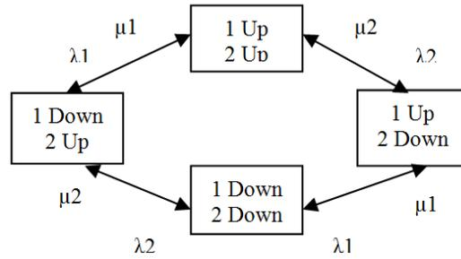
Figure 4: Model for overlapping independent outages of two components.
